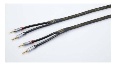
Speaker cables must be low-loss, which also relates to the damping factor of the driving amplifier. That's why the "Diamond 3" is at least twelve millimeters thick on the outside and has four strong stranded conductors made of 4VRC special copper conductors. Naturally, this also favors the offer for bi-wiring variants. With a full cross-section, the DC resistance is only 7.4 ohms per kilometer. With 750 € high sound value for the money! Clearly here too: **High End**.
