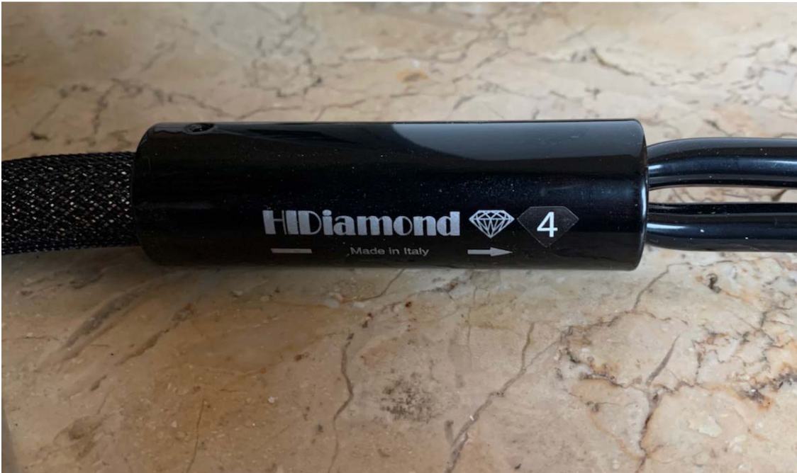
The flexible cables also have a marking of the signal direction
