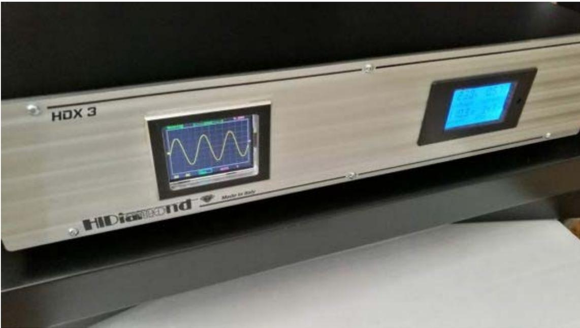
The 430mm wide (rack-sized) aluminum front panel, enclosed in a steel housing, is now standard in appearance and fits in with the overall design of our sound system. Here you like the front panel machining, the systematically arranged microbreaks provide a pleasant look.
