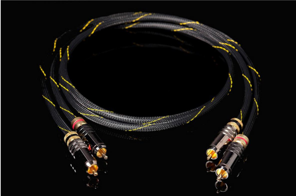
A Diamond 2, which is the second in the hierarchy, has 7mm outer diameter. The structure of cable is the same than above, but the declared capacitance is 114 pF/m, and the resistance of conductors is less, only 4,95 ohm/100m.
